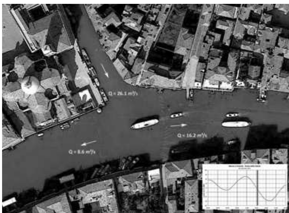
Fig. 2 - Flow measurements at the intersection of the Grand Canal-Cannaregio Canal near San Geremia church, carried out on 26/11/2011 during an ebb tide between 15.06 and 15.17. In the three sections of the node, measurements are not simultaneous, hence continuity cannot be rigorously respected.
