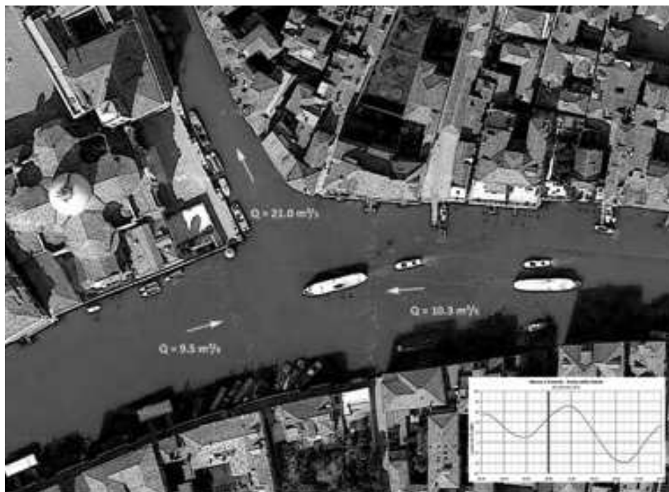
Fig. 1 - Flow measurements at the intersection of the Grand Canal-Cannaregio Canal near San Geremia church, carried out on 26/11/2011 during a flow tide between 8.57 e le ore 9.06. In the three sections of the node, measurements are not simultaneous, hence continuity cannot be rigorously respected.
